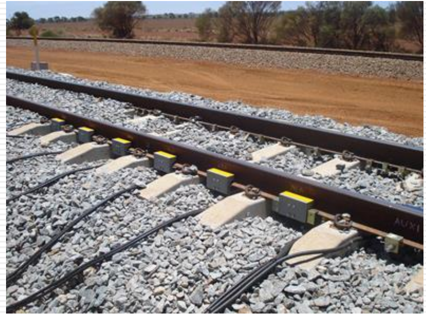
Wheel Condition Monitor from Track IQ
