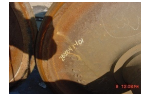
Cracked Wheel Plate
