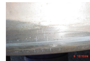
Tread Thermal Cracks
