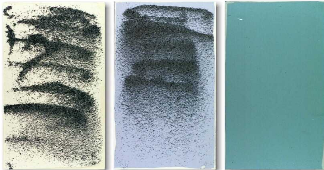
Blast Grit Applied 30 Minutes After Application
