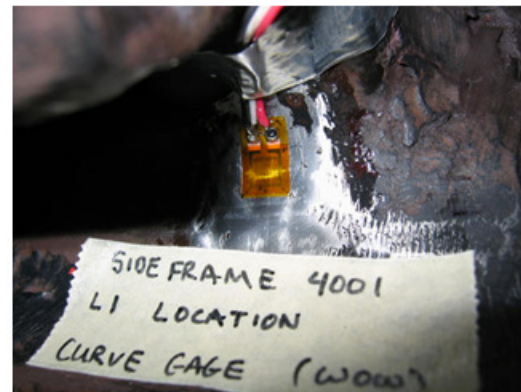
Figure 2: Location L1 curve location (left), strain gage installation at L1 (right)
