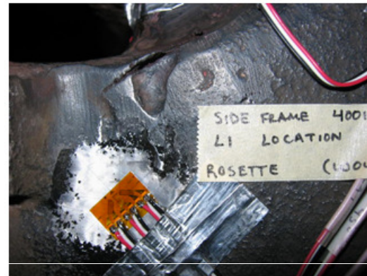
Figure 1: Location L1 side view (left) strain gage installation at L1 (right)
